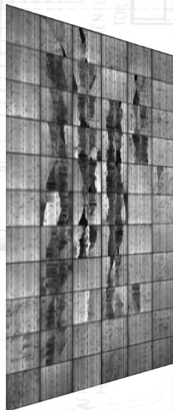
Panel with cell cracks
